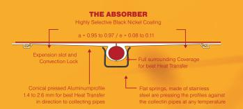
The secret for the excellent efficiency of the EKS solar collectors lies in the unique system of the absorbers with their conical pressed aluminium profiles, their spring loaded covers for the copper tubes and their lock against air convection. Therefore the maximum efficiency is approximately 87 %, in relation to the absorber area.
